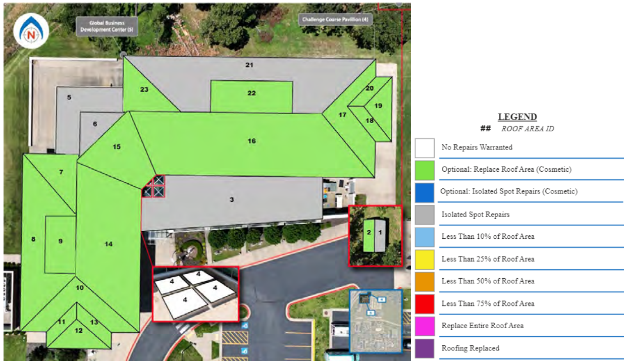
Figure 103. Excerpt of SAM Q-PDF® that depicts the minimum roofing repairs by color.
