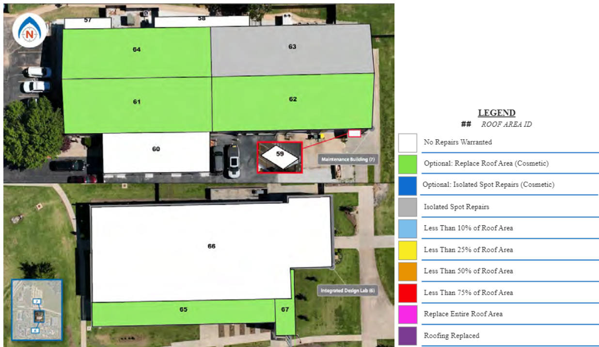
Figure 104. Excerpt of SAM Q-PDF® that depicts the minimum roofing repairs by color.
