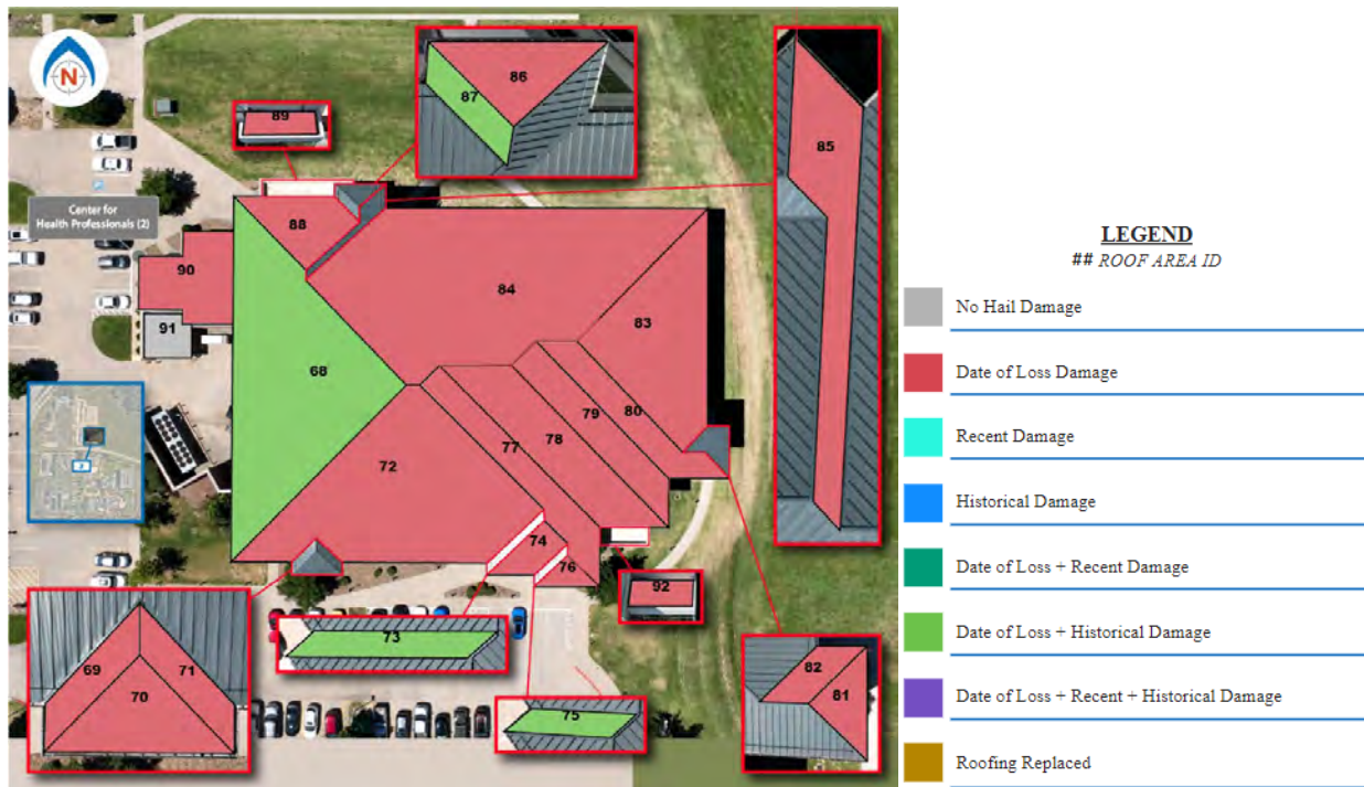
Figure 5. Excerpt of SAM Q-PDF® that depicts the locations and relative date(s) of occurrence of hail-related conditions to the roofing, by color.
