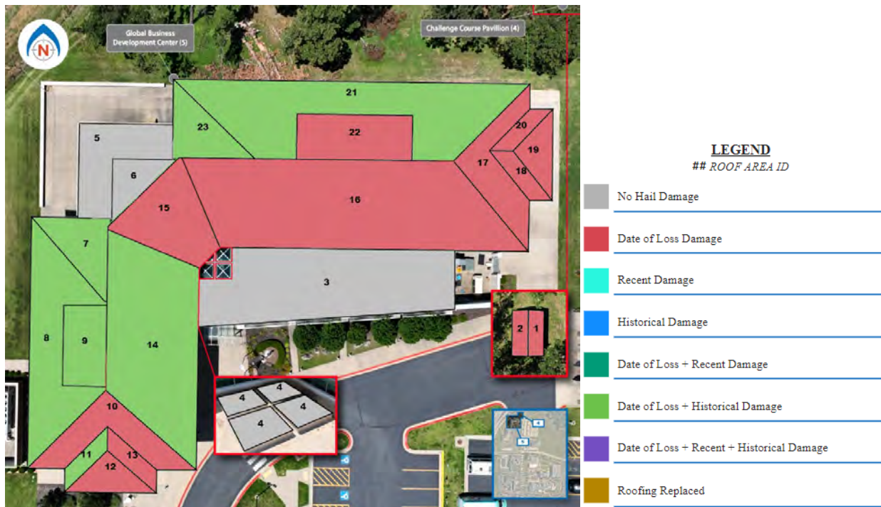
Figure 7. Excerpt of SAM Q-PDF ® that depicts the locations and relative date(s) of occurrence of hail-related conditions to the roofing, by color.
