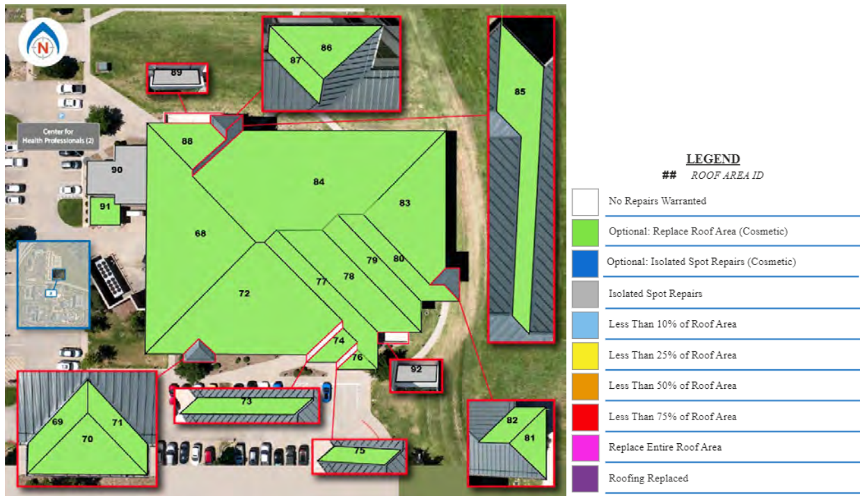
Figure 101. Excerpt of SAM Q-PDF ® that depicts the minimum roofing repairs by color.
