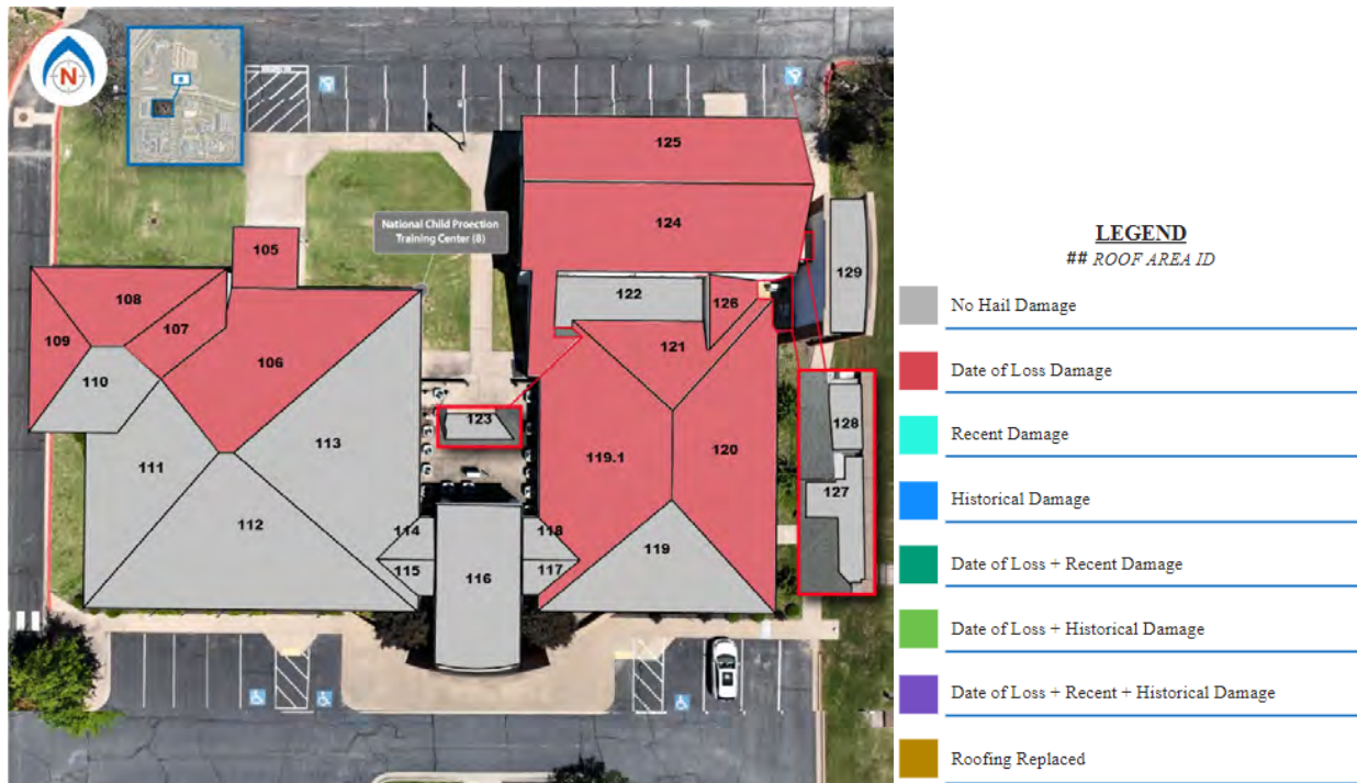
Figure 9. Excerpt of SAM Q-PDF® that depicts the locations and relative date(s) of occurrence of hail-related conditions to the roofing, by color.
